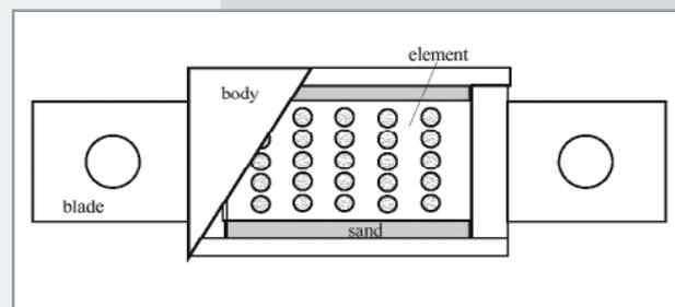
Figure 3: Cut away view of short circuit element
