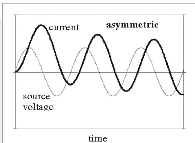
Figure 2: Typical short circuit current waveform
