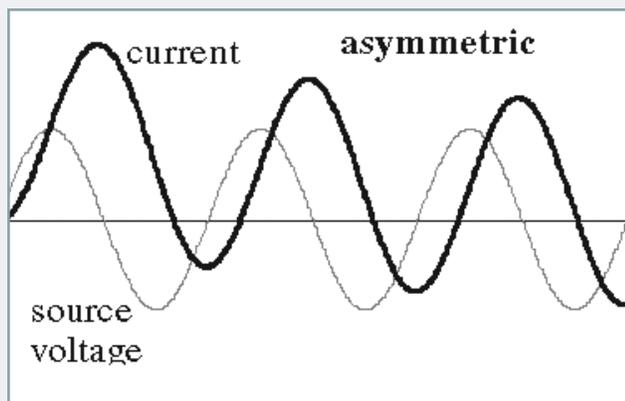
Figure 6: Asymmetrical current waveform
