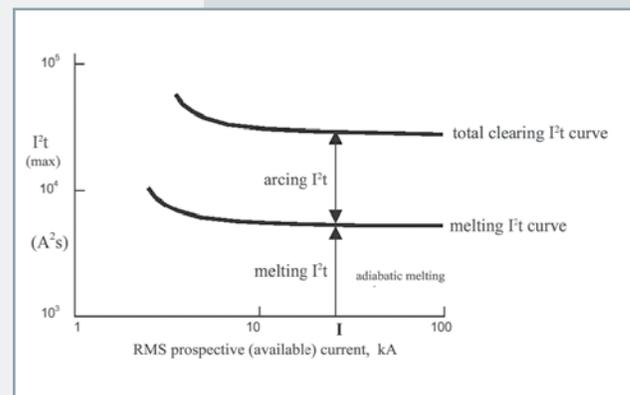
Figure 8:  $I^2t$  versus available fault current
