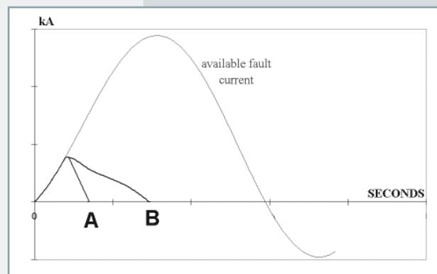
Figure 5: Clearing time effects on  $I^2t$
