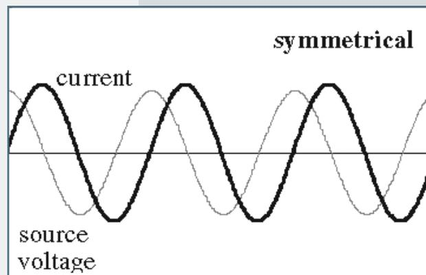
Figure 7: Symmetrical current waveform
