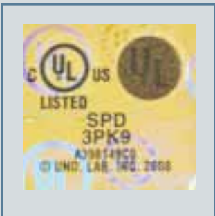
Figure 3: The above picture is of a holographic label from a UL 1449 3rd Edition device. Please note the SPD wording, which is accepted in today's industry.
