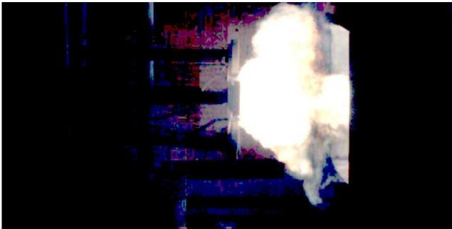
Fig. 4 Plasma Development With Insulating Barrier
