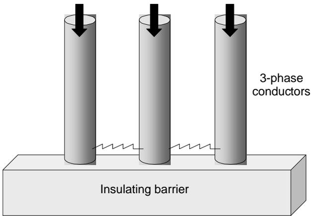
Fig. 1 Test Electrodes Terminated with Insulating Barrier
