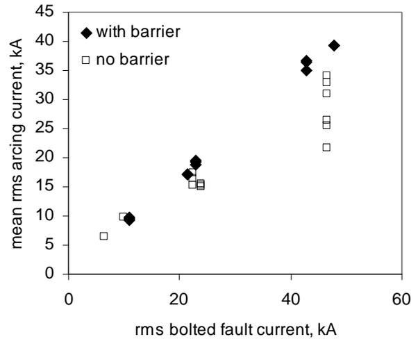
Fig. 2 Effect of Barrier on Mean Arcing Current
