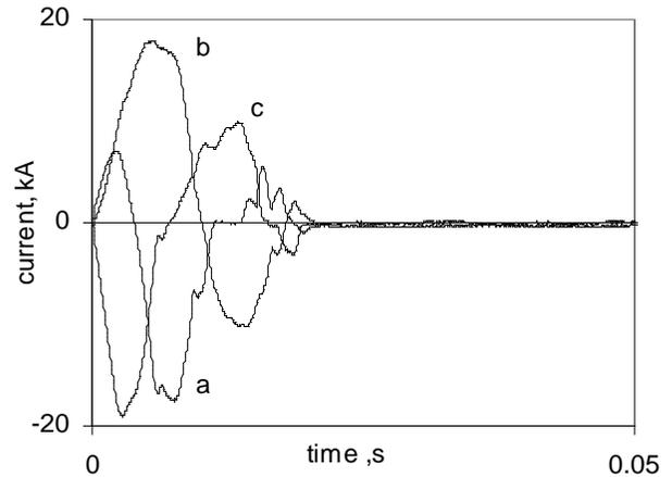
Fig. 6 Arcing Currents at 250V, 13kA - No Barrier
