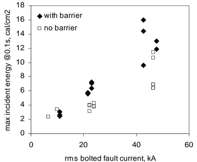
Fig. 3 Effect of Barrier on Incident Energy Density
