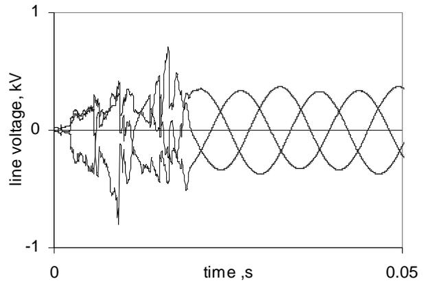
Fig. 7. Line-line Voltages at 250V, 13kA - No Barrier
