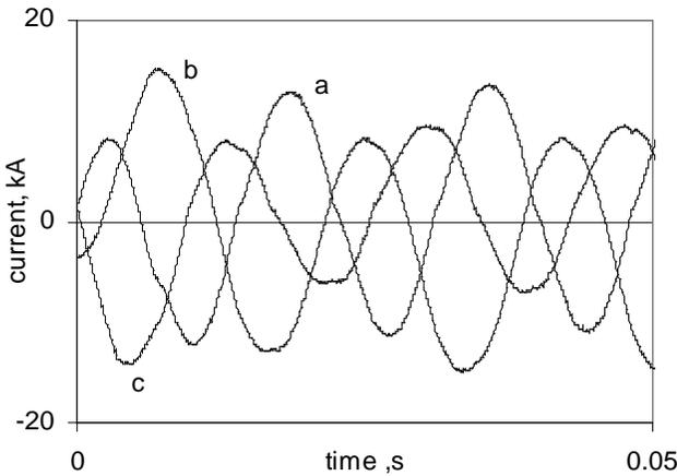
Fig. 8 Arcing Currents at 208V, 9.9kA - With Barrier
