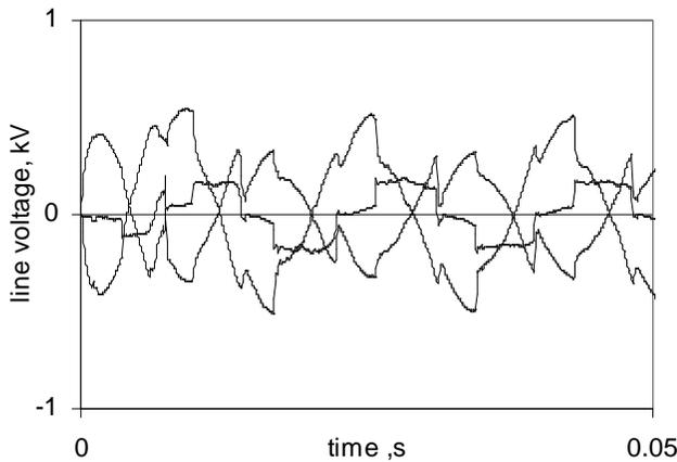
Fig. 9. Line-line Voltages at 208V, 9.9kA - With Barrier
