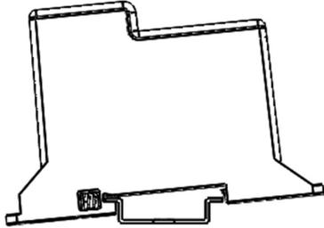
1. Hook line side over 35mm DIN Rail
